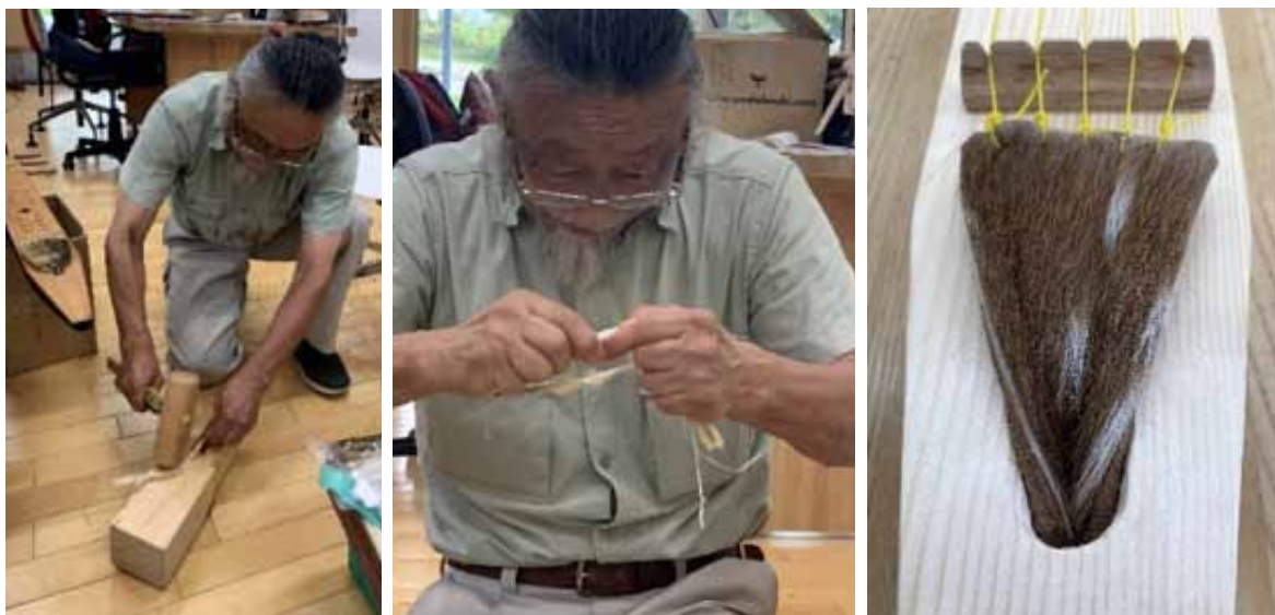
Figure 6. Left, Takano Shigehiro demonstrated pounding & crushing deer Achilles tendon. Center, the process of braiding deer Achilles tendon for musical instrument strings. Right, Seal skin is used as neo [cloth end piece anchoring the strings. Photos by the author.
